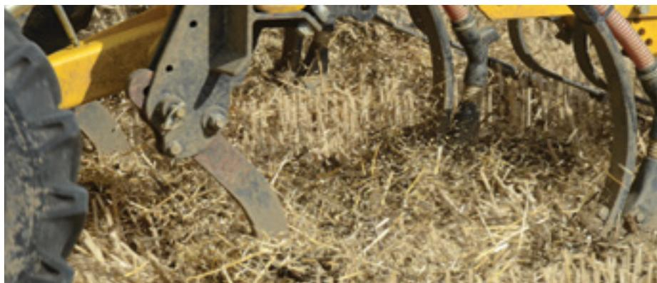
**Leading tines can be adjusted to stimulate the soil to the required rooting depth, from 0cm down to 15cm for deep rooting crops such as oilseed rape. Rick Davies operates them at 12.5cm for the majority of situations, while adjusting the seeding tine as shallow or deep as necessary.**
